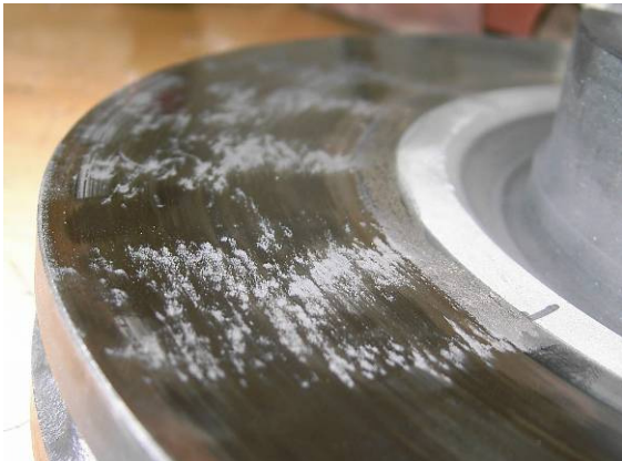
Figure 8: Manipulated disk with deep grooves after heavy braking
