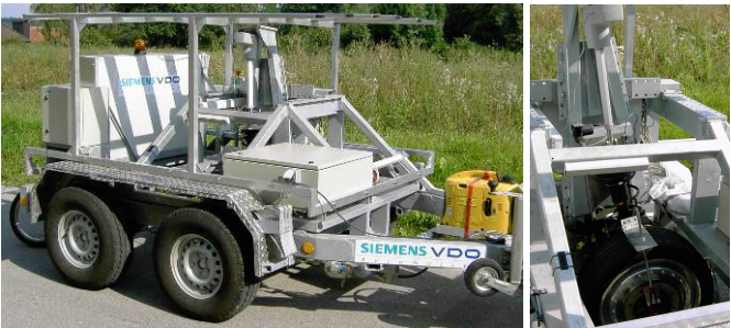
Figure 3: Mobile quarter vehicle test rig
