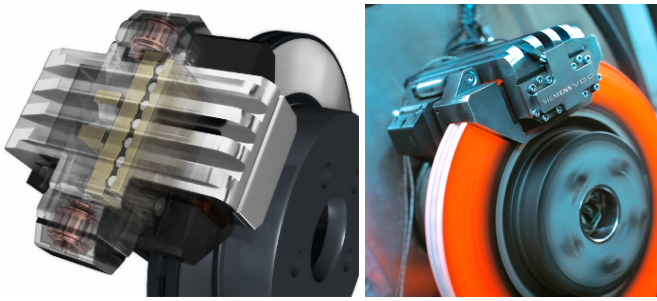
Figure 1: Beta prototype with full functionality, wedge bearing in detail (left), and high temperature test with optimized heat dissipation (right)
